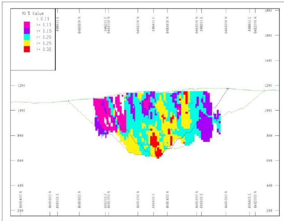
Figure 16.8 Block Model - Ni values - Section SE\_21 Looking NW
